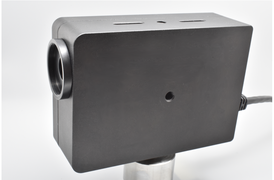
A Crunch Cam module, which acquires and processes beam image data.
